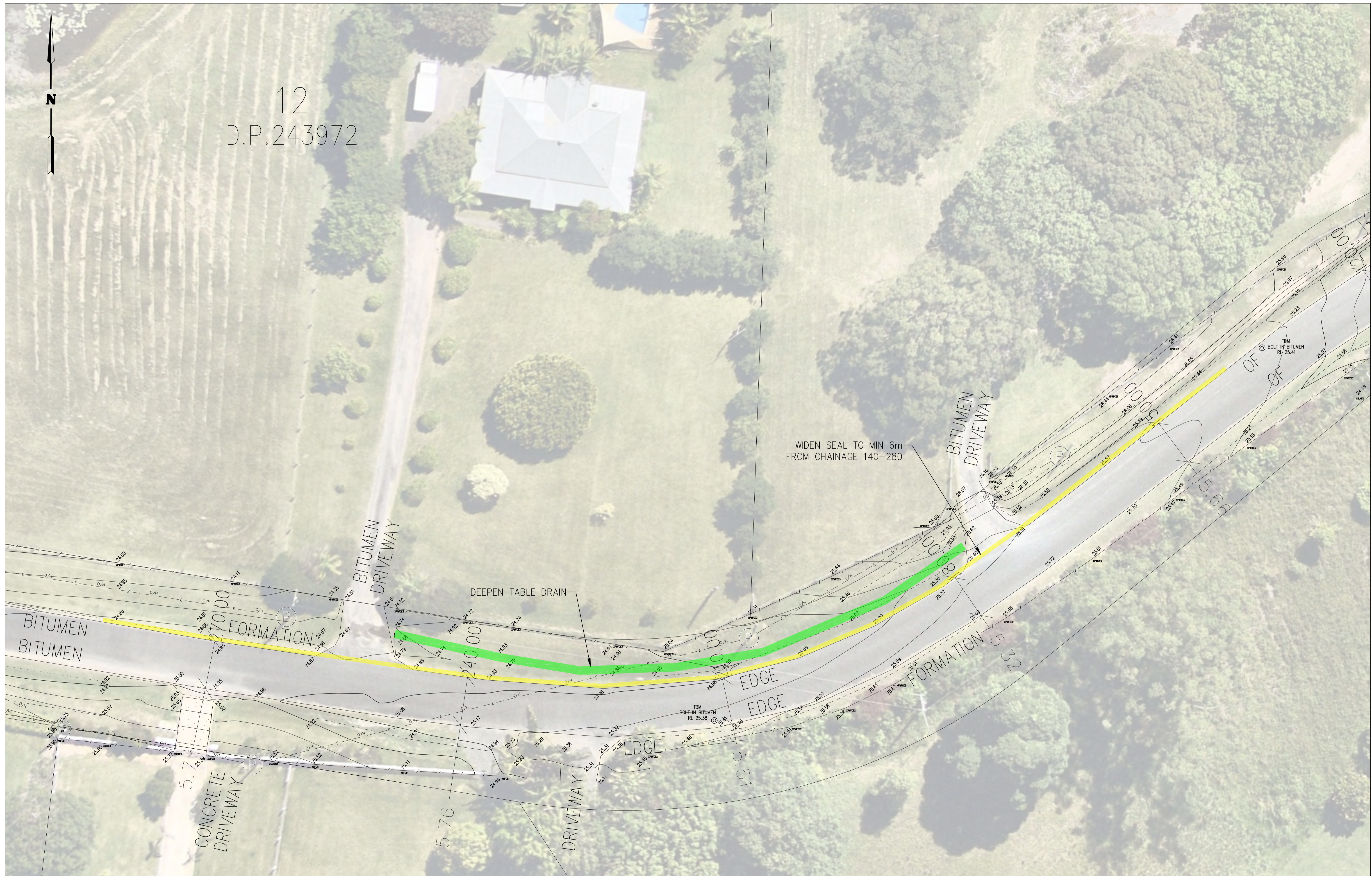
RECOMMENDED PAVEMENT WIDENING, SUGAR MILL ROAD
